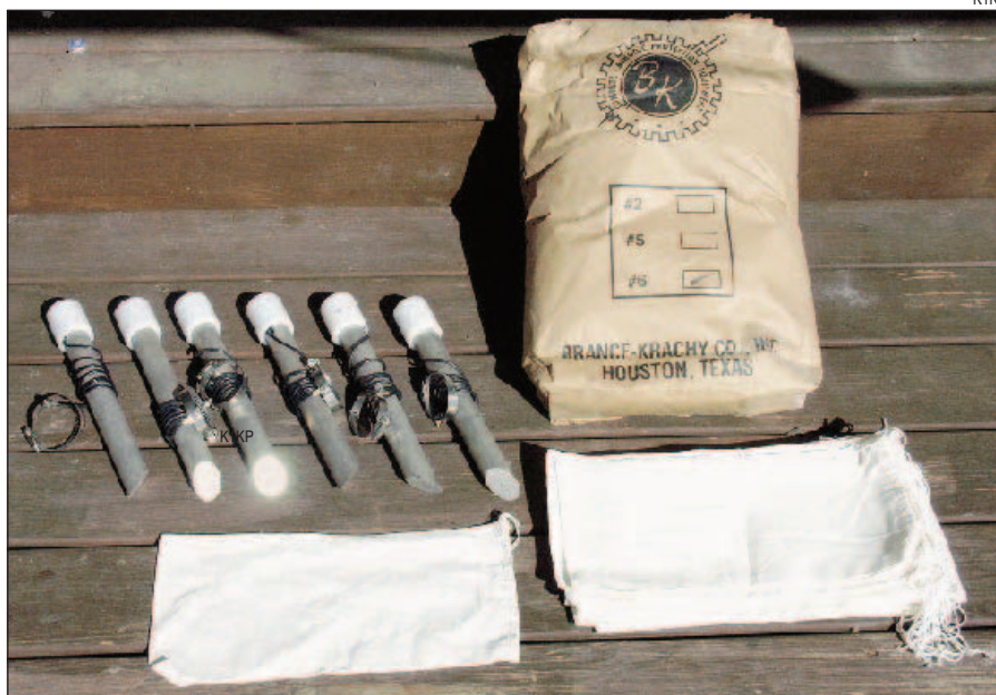
Figure 4 — All the materials required to build six sacrificial anodes.
