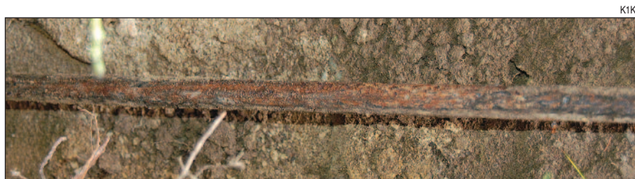
Figure 2 — Guy anchor rod inspection. This rod has lost all of its galvanized coating, exposing the steel to corrosion.
